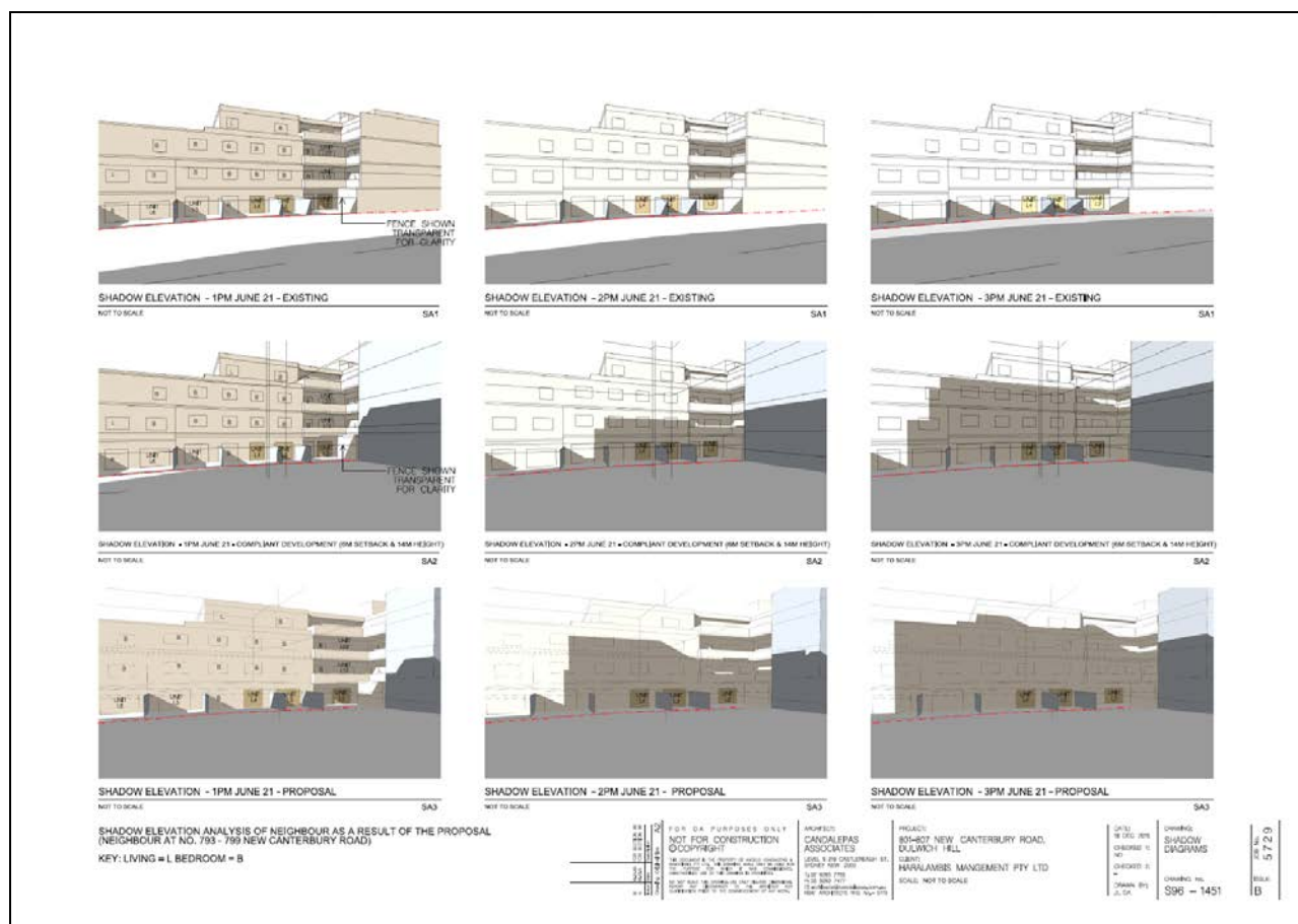
Image 19: Elevational shadow analysis for the Section 96 application (Scenarios SA1-SA3)**
